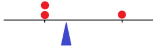
Intuitively we expect the balance point of this system to be closer to the two marbles than the single one. How much closer?
