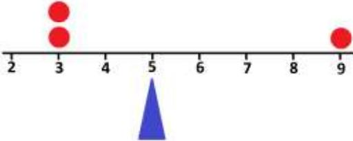
By Archimedes Law of the Lever, the balance point of this system occurs one-third of the way between locations 3 and 9, namely at 5.
