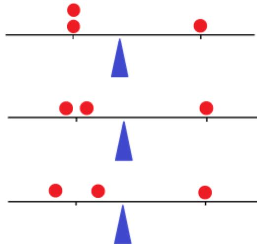
Keep teasing the two marbles apart until we have three equally spaced marbles. The balance point of the system still has not changed.
