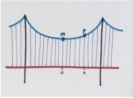
We'll assume the weights of vertical cables and the main suspension cable are negligible compared to the weight of the road. We'll also assume that the spacing of the vertical cables is quite dense along the length of the road in the sense that every point on the suspension cable is very close to a vertical cable.
