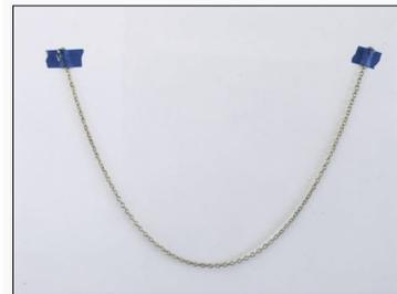
c) The shape of a hanging chain being used to support a linear stretch of road beneath it, as for a classic suspension bridge.
